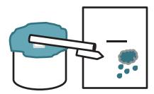
When the ambient or surrounding pressure increases or becomes higher than the inside of the jar, the balloon will be pushed down making the straw tilt upward below the reference line. This indicates dry and cool weather is coming.
